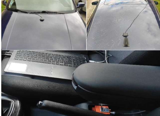
Fig.2. Position of GNSS antennas (Top), position of inertial measurement unit (Bottom).
