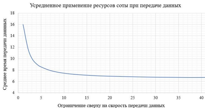
Fig.9. Average use of cell resources in data transmission, in case when maximum resources are available for data traffic.
