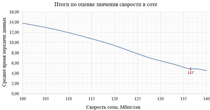
Fig.2. Estimates of the rate in the cell, which will allow the processing of requests for all types of traffic, with permissible losses and average transmission time.
