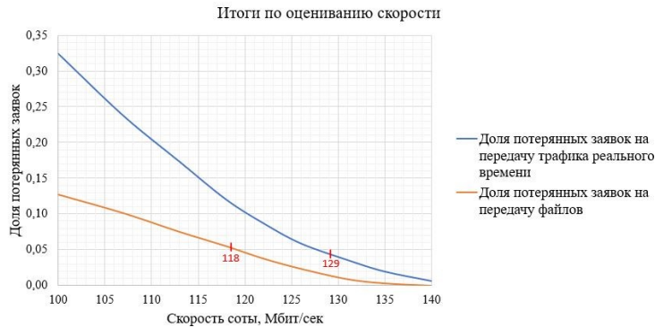
Fig.1. Results on estimation of the rate at which the transmission takes place in the part of the LTE network at which requests for all types of traffic can be processed, with the limit loss value.
