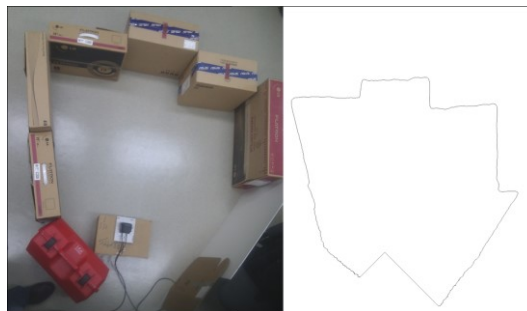
Fig.6. Artificially made environment (left) and its local map (right).
