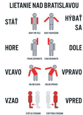
Figure 2: Manual sheet with the gestures and postures for navigating in the 3D world.
