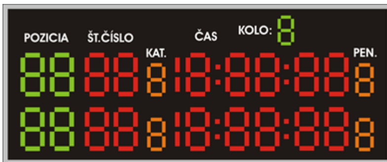
Figure 3. Design of 7 segment outdoor display, from left to right: rank, starting number, category, time, round, penalisation.
